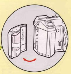
Load the lithium battery inside the battery grip, and replace the battery grip.
