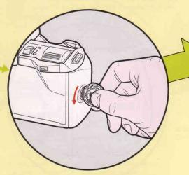
Remove the battery grip by turning the screw counter-clockwise with a coin.
